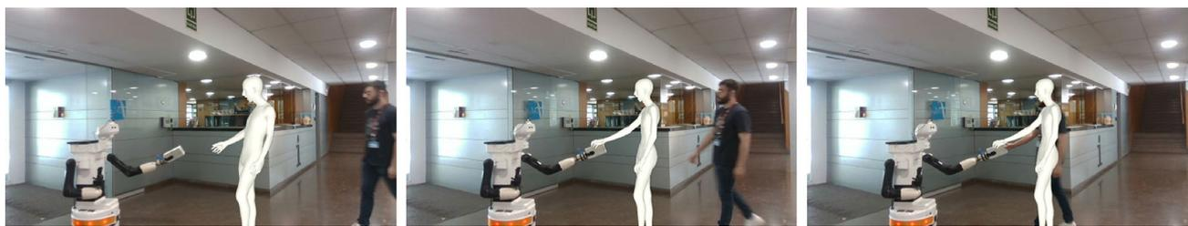
**Fig. 1** Visual representation of the prediction being used by the robot. We utilized the SMPL parametric model [1] to provide a realistic visualization of the 3D human body of the user during a human–robot handover. In the final frame, the user reached a close position with respect to the predicted pose
