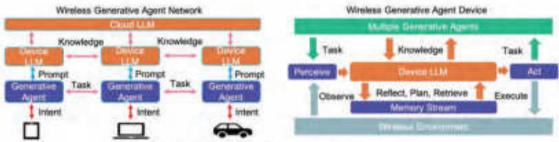
Fig. 2: Wireless generative agent network and device architecture,
